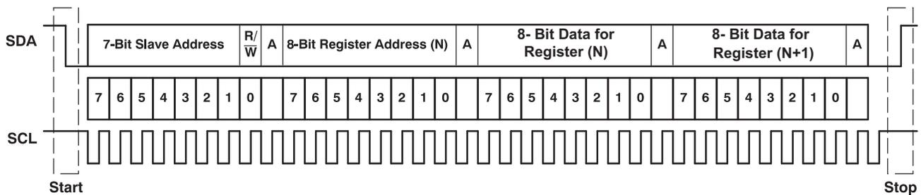
**Figure 5. Typical I<sup>2</sup>C Sequence**
