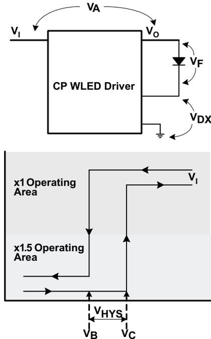
Figure 13. Input Voltage Hysteresis Between 1x and 1.5x Mode
