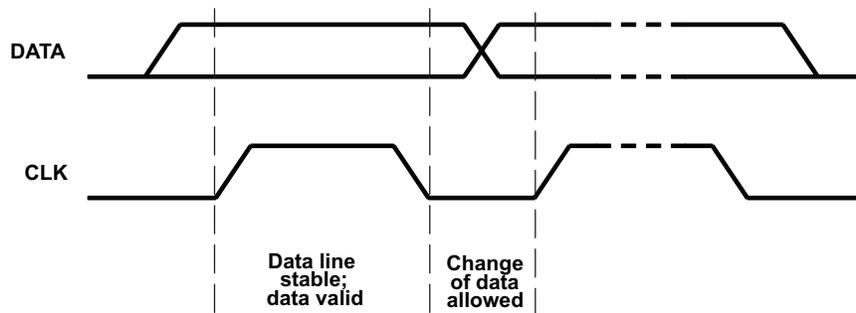
Figure 15. Bit Transfer on the Serial Interface
