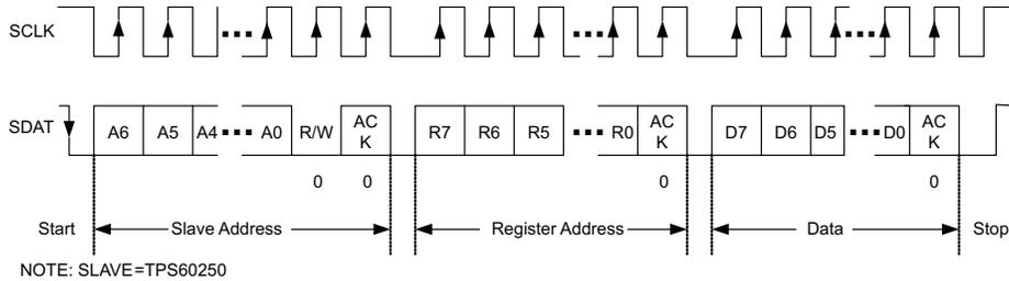
Figure 17. Serial I/F READ From TPS60250: Protocol A
