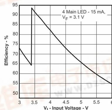
Figure 2. Efficiency vs Input Voltage
