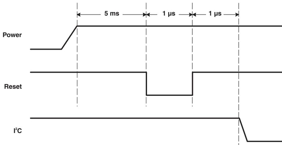
**Figure 7. Reset Timing**
