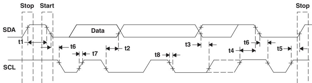
**Figure 2. I<sup>2</sup>C Host Port Timing**
