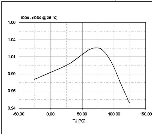
Figure 11. Operating supply current (switching) vs  $T_J$
