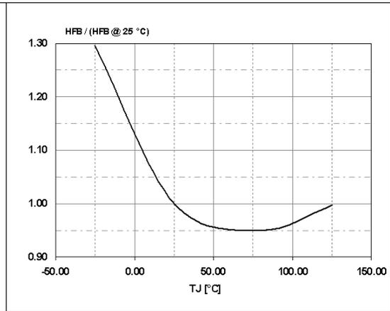
Figure 10. Operating supply current (no switching) vs  $T_J$
