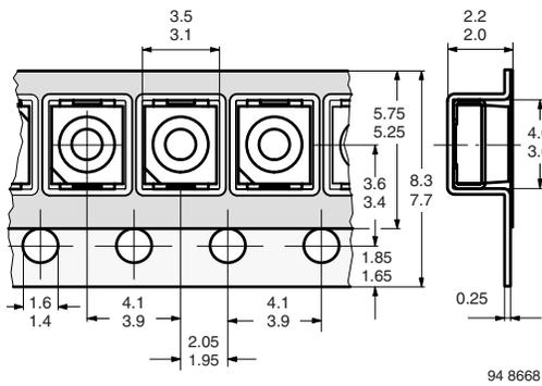
Figure 11. Tape Dimensions in mm for PLCC-2
