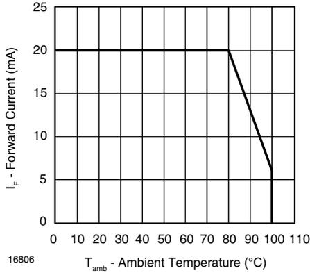
Figure 1. Forward Current vs. Ambient Temperature for InGaN
