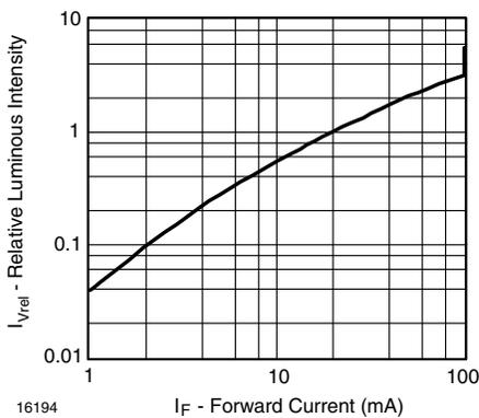
Figure 3. Specific Luminous Flux vs. Forward Current
