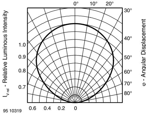
Figure 2. Relative Luminous Intensity vs. Angular Displacement
