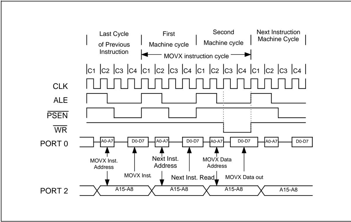
Figure 8. Data Memory Write with Stretch Value = 0
