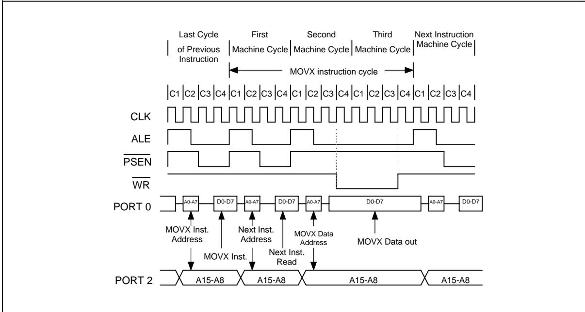
Figure 9. Data Memory Write with Stretch Value = 1
