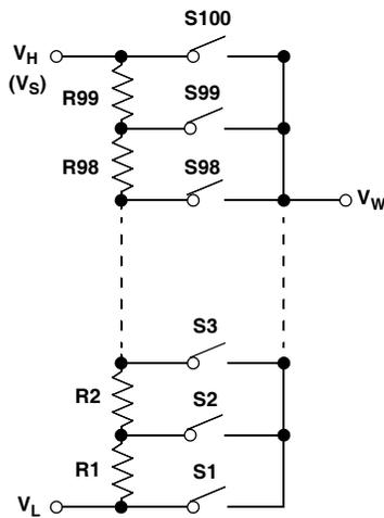
$$G_i = 20 \text{Log} \frac{R_1 + R_2 + \dots + R_i}{R_{\text{TOTAL}}} = \frac{V_W}{V_S} (V_L = 0V)$$
