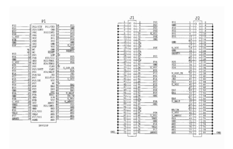
Figure 1. Schematic for Z89323 68-pin PLCC Emulation Pod
