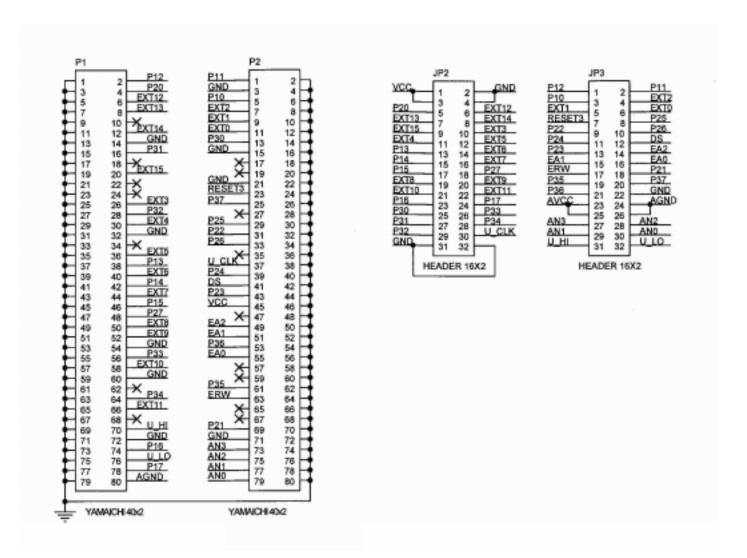
Figure 2. Schematic for Z89323 Emulation Pod Adapter
