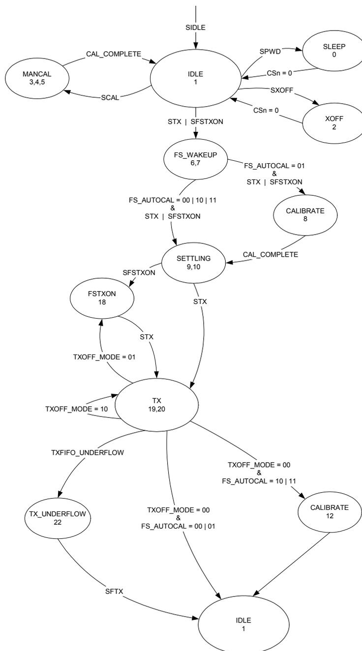
**Figure 10: Radio Control State Diagram**
