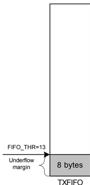
Figure 13: Example of FIFO at threshold
