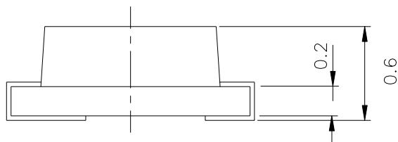
For reflow soldering (Propose)
