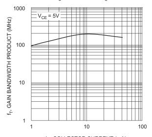
$\rm I_{\rm C}$ , COLLECTOR CURRENT (mA) Fig. 3, Gain Bandwidth Product vs Collector Current
