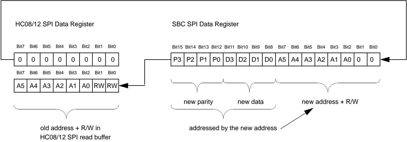
**Figure 20. Microcontroller SPI Reading Data - Sequence B**
