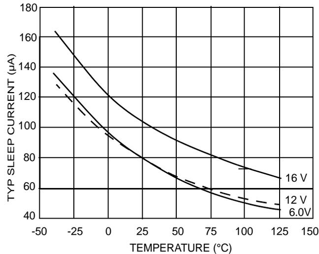
Figure 15. Current vs Temp and Batt Voltage
