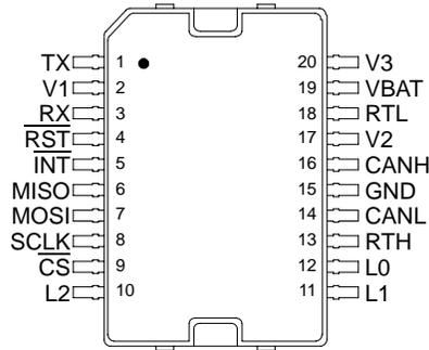
Figure 3. 33389 Pin Connections
