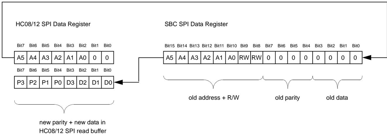
Figure 21. Microcontroller SPI Reading Data - Sequence C
