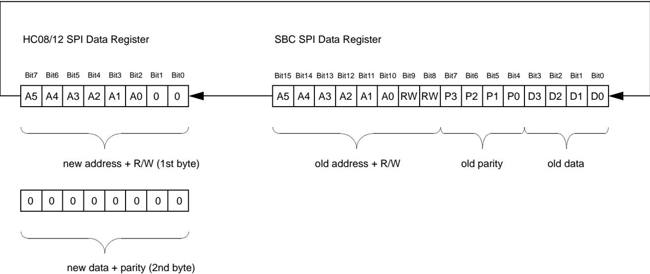
**Figure 19. Microcontroller SPI Reading Data - Sequence A**
