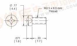
Material: Steel Plating: Zinc Thread Size: M2.5 Package Size: 200 Pieces
