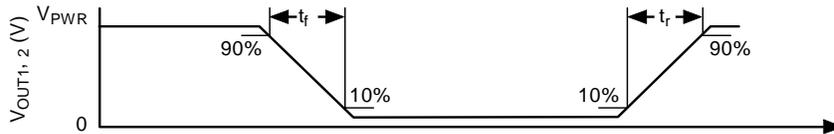
Figure 6. Output Switching Time
