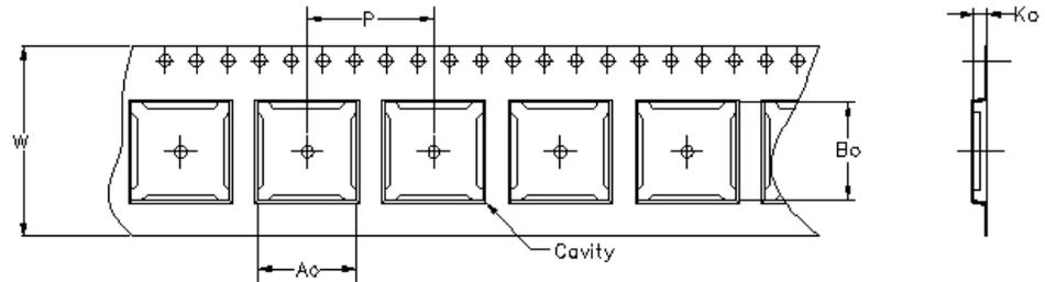
Carrier tape design is defined largely by the component length, width, and thickness.
