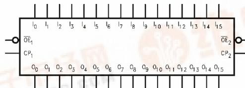
74VCX16374 Low Voltage 16-Bit D-Type Flip-Flops with 3.6V Tolerant Inputs and Outputs
