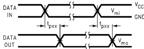
**FIGURE 8. Waveform for Inverting and Non-Inverting Functions**
