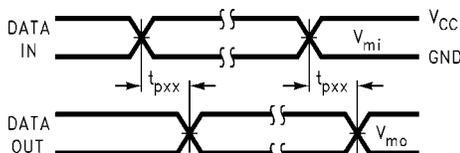
FIGURE 2. Waveform for Inverting and Non-Inverting Functions
