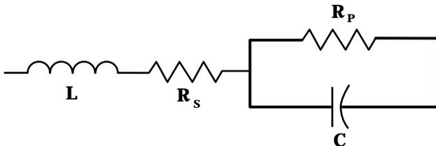
**Reactance** – Since the insulation resistance (**R<sub>p</sub>**) is normally very high, the total impedance of a capacitor is:
