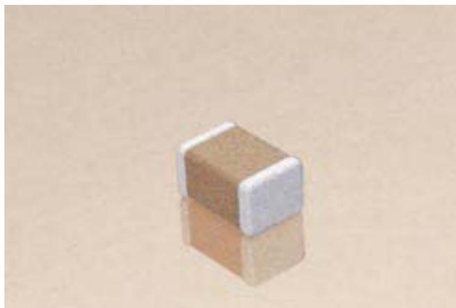
X7R formulations are called “temperature stable” ceramics and fall into EIA Class II materials. X7R is the most popular of these intermediate dielectric constant materials. Its temperature variation of capacitance is within  $\pm 15\%$  from  $-55^{\circ}\text{C}$  to  $+125^{\circ}\text{C}$ . This capacitance change is non-linear.
