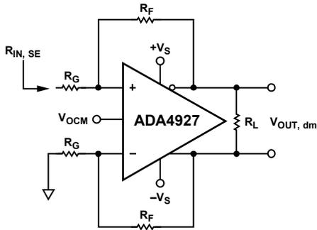
Figure 49. The ADA4927 with Unbalanced (Single-Ended) Input
