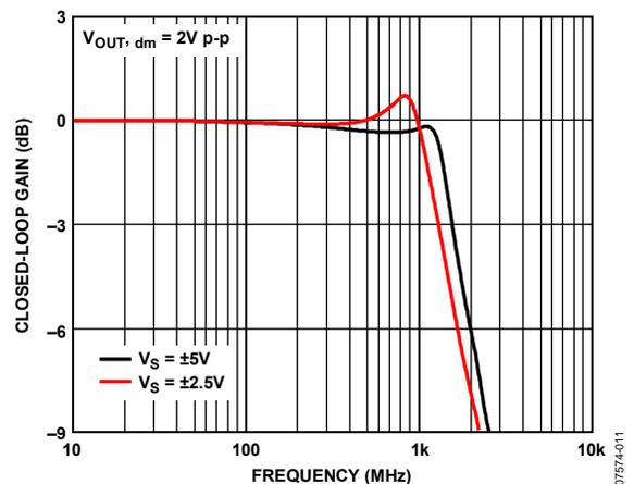
Figure 11. Large Signal Frequency Response for Various Supplies
