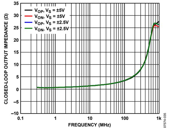
Figure 35. Closed-Loop Output Impedance Magnitude vs. Frequency at Various Supplies,  $G = 1$
