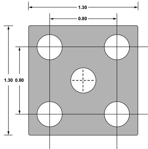
Figure 56. Recommended PCB Thermal Attach Pad Dimensions (Millimeters)
