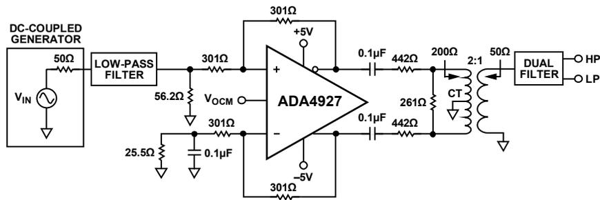
Figure 45. Test Circuit for Distortion Measurements
