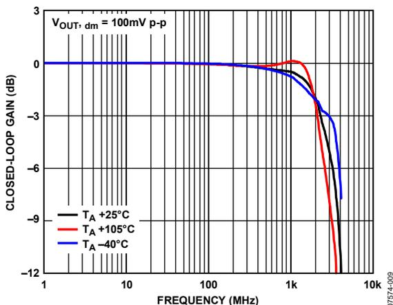
Figure 9. Small Signal Frequency Response for Various Temperatures
