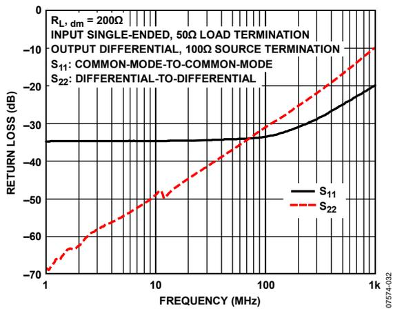
Figure 32. Return Loss ( $S_{11}$ ,  $S_{22}$ ) vs. Frequency
