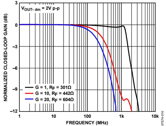
Figure 10. Large Signal Frequency Response for Various Gains
