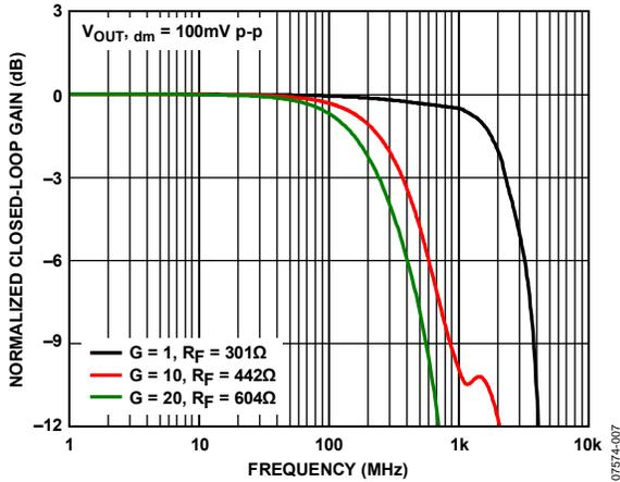
Figure 7. Small Signal Frequency Response for Various Gains
