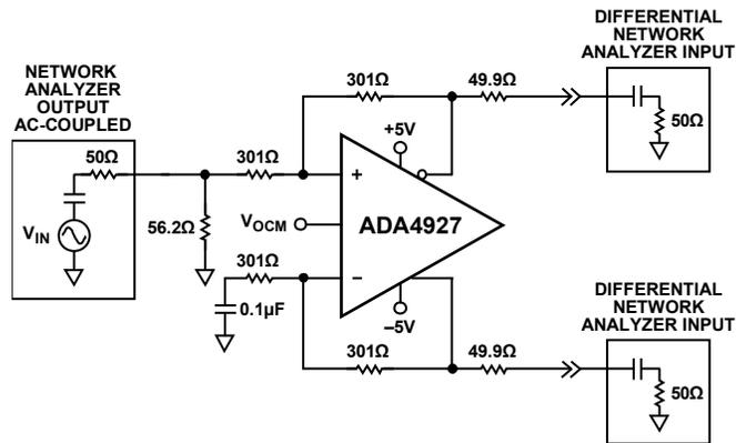
Figure 44. Test Circuit for Output Balance, CMRR
