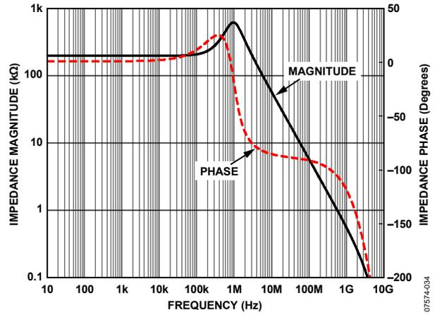
Figure 34. Open-Loop Transimpedance Magnitude and Phase vs. Frequency
