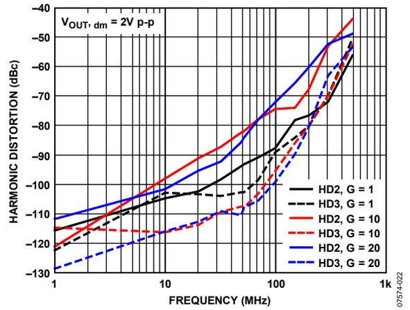
Figure 22. Harmonic Distortion vs. Frequency at Various Gains
