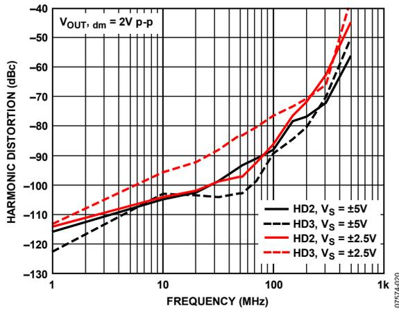
Figure 20. Harmonic Distortion vs. Frequency at Various Supplies
