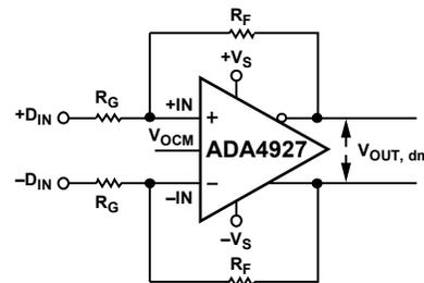
Figure 48. The ADA4927 Configured for Balanced (Differential) Inputs
