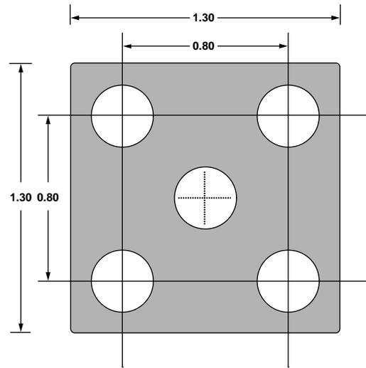
Figure 65. Recommended PCB Thermal Attach Pad Dimensions (Millimeters)
