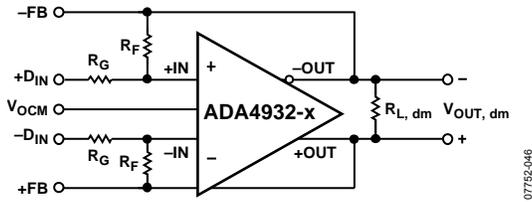
Figure 55. Signal and Circuit Definitions
