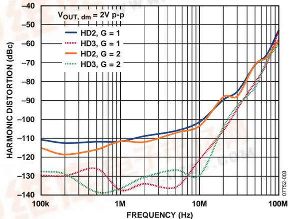
Figure 3. Harmonic Distortion vs. Frequency at Various Gains
