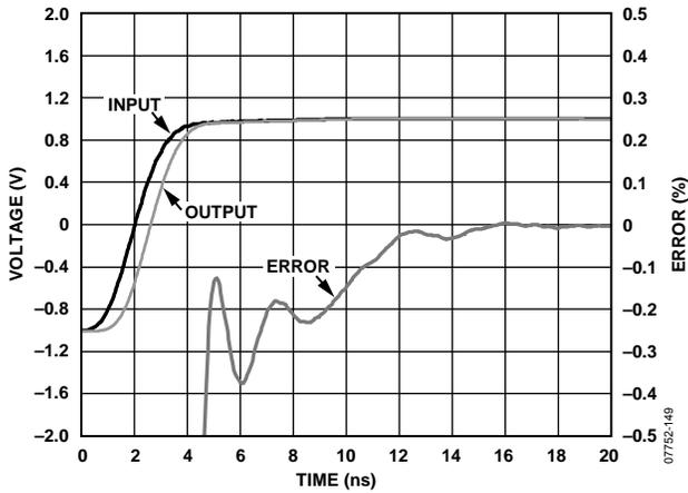
Figure 49. Settling Time
