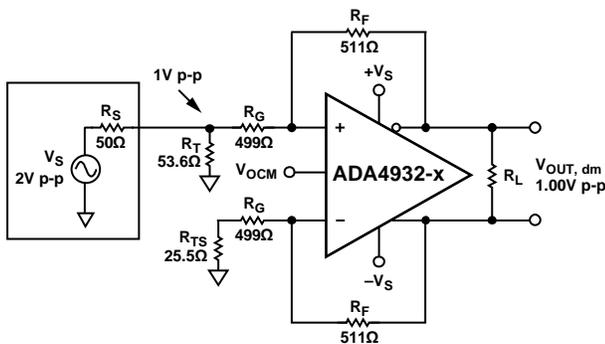
Figure 63. Terminated Single-Ended-to-Differential System with  $G = 2$
