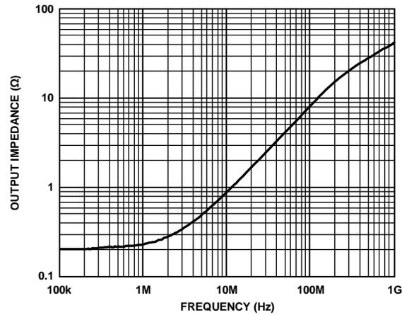
Figure 41. Closed-Loop Output Impedance Magnitude vs. Frequency,  $G = 1$
