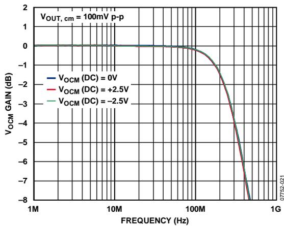
Figure 21.  $V_{OCM}$  Small Signal Frequency Response at Various DC Levels
