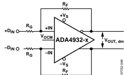
Figure 57. ADA4932-x Configured for Balanced (Differential) Inputs
