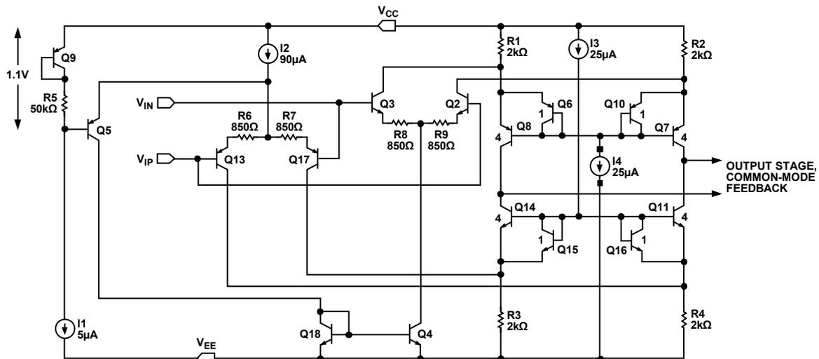
Figure 43. Simplified Schematic of AD8031 Input Stage
