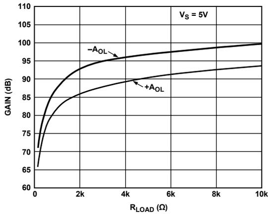
Figure 20. Open-Loop Gain ( $A_{OL}$ ) vs.  $R_{LOAD}$
