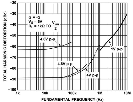
Figure 31. Total Harmonic Distortion vs. Frequency;  $G = +2$
