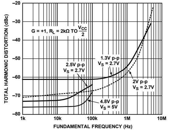
Figure 30. Total Harmonic Distortion vs. Frequency;  $G = +1$
