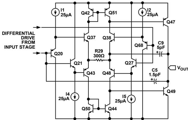
Figure 44. Output Stage Simplified Schematic
