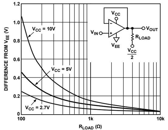
Figure 18. -Output Saturation Voltage vs.  $R_{LOAD}$  @ +25°C
