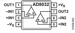
Figure 2. 8-Lead PDIP (N), SOIC\_N (R), and MSOP (RM)
