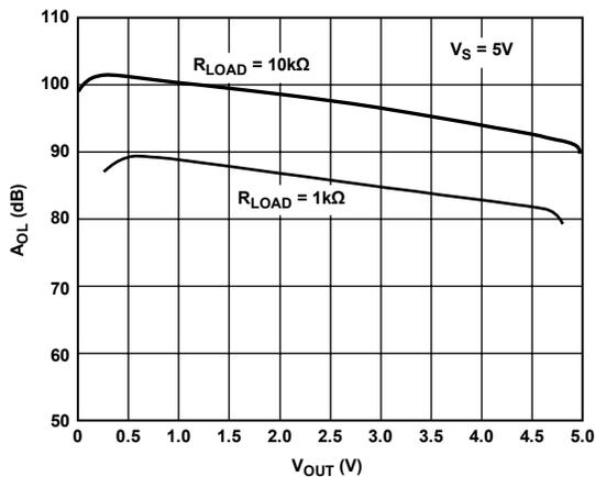
Figure 22. Open-Loop Gain ( $A_{OL}$ ) vs.  $V_{OUT}$
