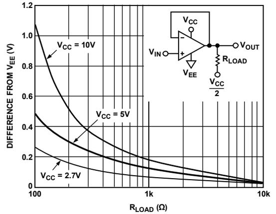
Figure 17. -Output Saturation Voltage vs.  $R_{LOAD}$  @ +85°C
