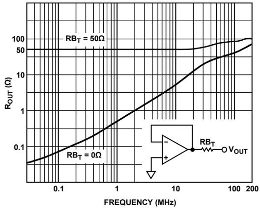
Figure 33.  $R_{OUT}$  vs. Frequency
