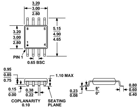
Figure 64. 8-Lead Mini Small Outline Package [MSOP]
