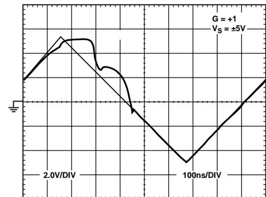
Figure 27. Input Overdrive Recovery (See Figure 42)
