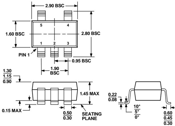
Figure 63. 5-Lead Small Outline Transistor Package [SOT-23]
