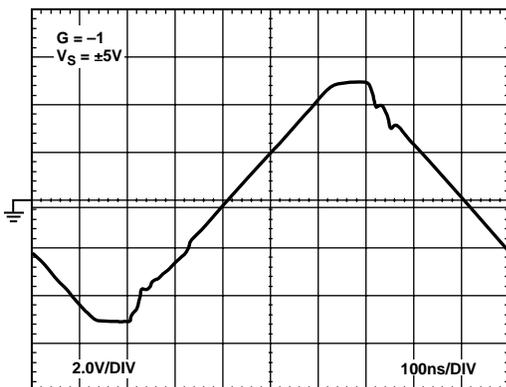
Figure 24. Output Overdrive Recovery (See Figure 44)
