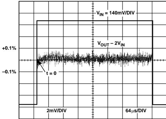
Figure 28. Long-Term Settling Time (See Figure 49)
