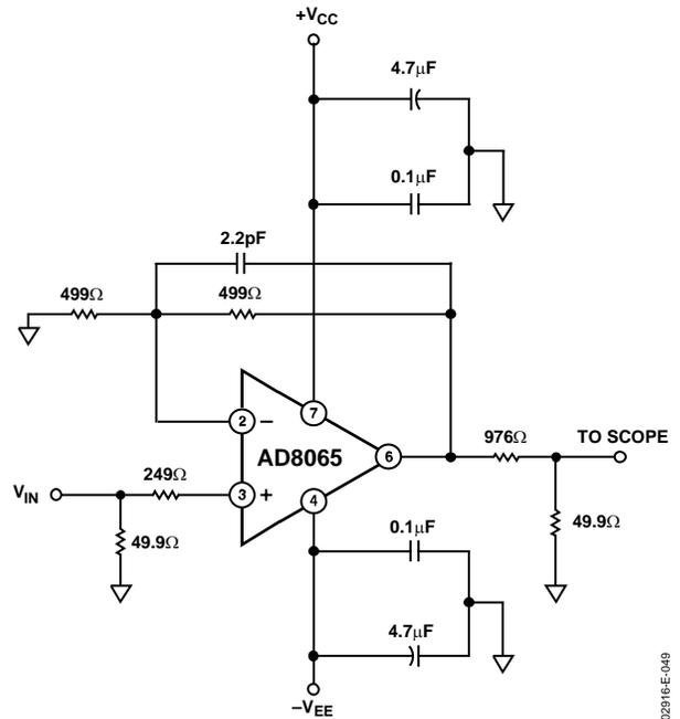
Figure 49. Settling Time
