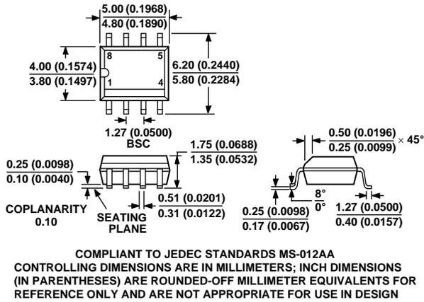
Figure 62. 8-Lead Standard Small Outline Package [SOIC]
