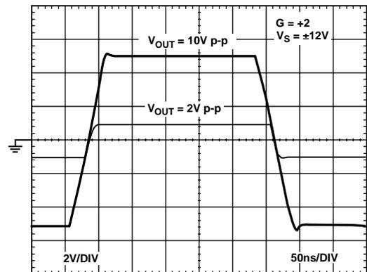
Figure 26. Large Signal Transient Response (See Figure 43)
