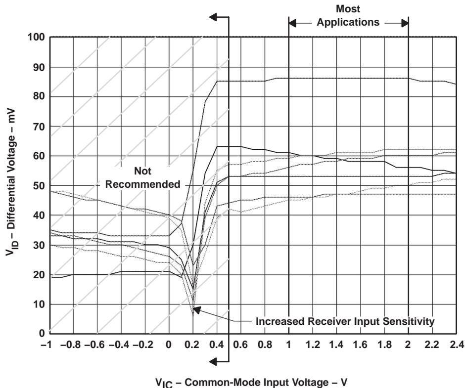
Figure 8.  $V_{IC}$  Versus  $V_{ID}$  Receiver Sensitivity Levels
