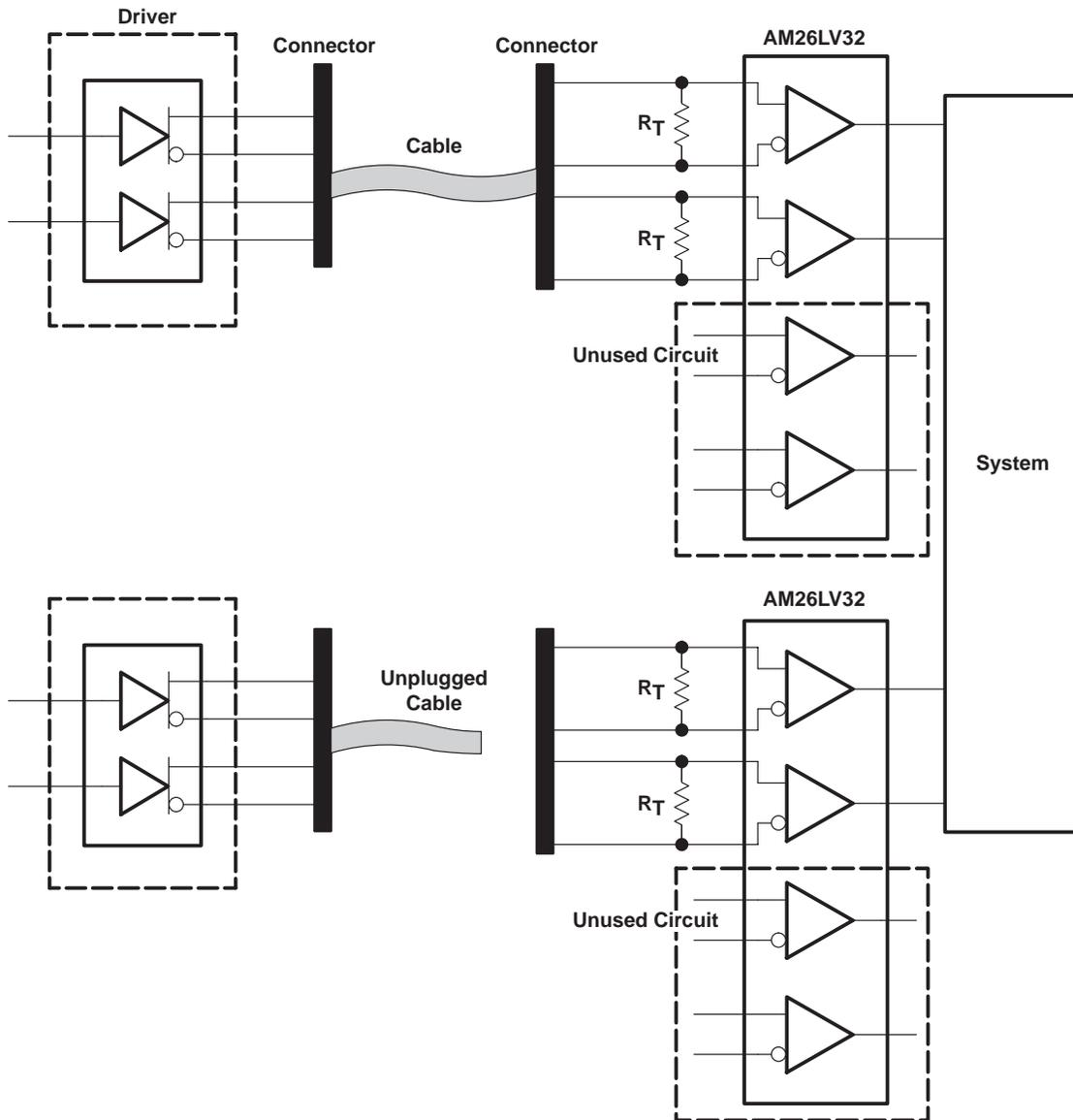
Figure 13. Alternative Solution to Figure 12
