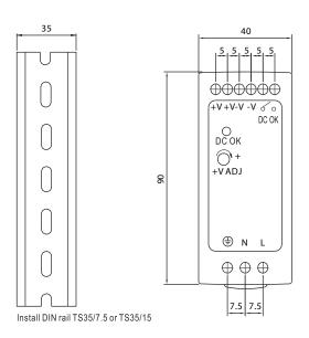
All dimensions shown in millimeters. To convert to inches multiply by 0.03937
