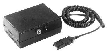
The MOD400R Field Sensitivity Test Module can be used with any standard DC voltmeter or multimeter to check the sensitivity range of System Sensor's detectors (satisfies NFPA 72 requirement for sensitivity testing).
