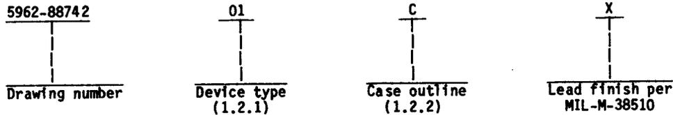
1.2.1 Device type. The device type shall identify the circuit function as follows:
