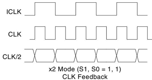
Using CLK as the feedback will always result in synchronized rising edges between ICLK and CLK. However, the CLK/2 could be a falling edge compared with ICLK. ICS recommends using CLK/2 feedback whenever possible. This will synchronize the rising edges of all three clocks.
