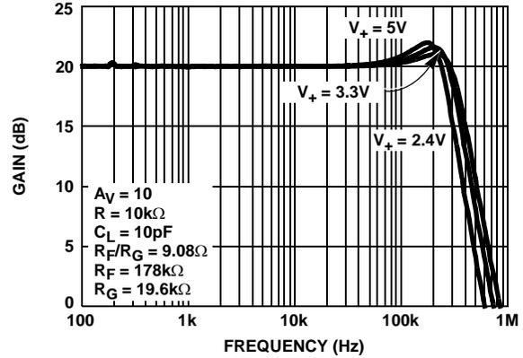
FIGURE 8. ISL28273 FREQUENCY RESPONSE vs SUPPLY VOLTAGE
