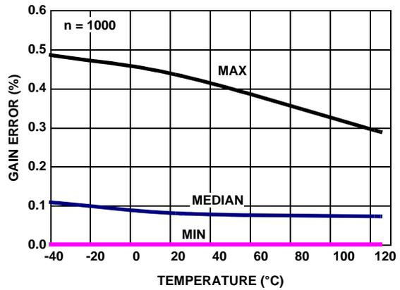
FIGURE 44. ISL28273 % GAIN ERROR vs TEMPERATURE,  $R_L = 100k$
