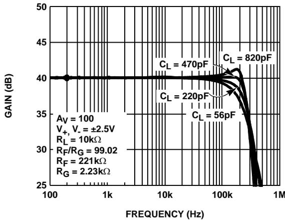
FIGURE 9. ISL28270, ISL28470 FREQUENCY RESPONSE vs  $C_{LOAD}$
