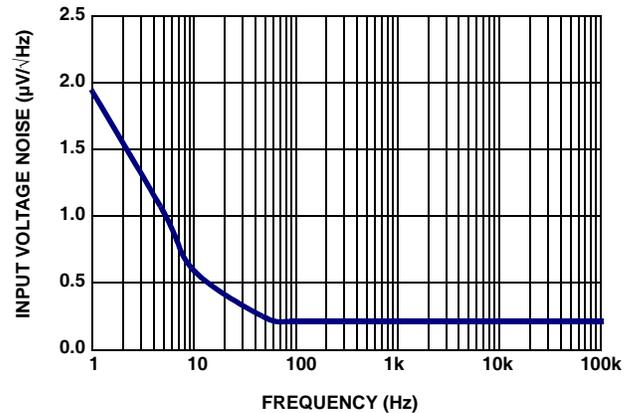
FIGURE 16. ISL28273 INPUT VOLTAGE NOISE SPECTRAL DENSITY (GAIN = 10)
