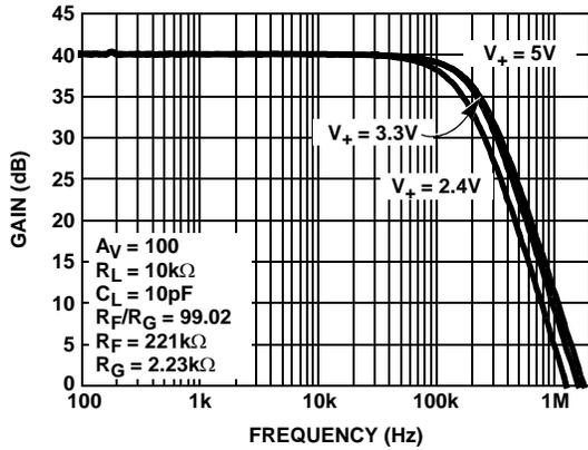
FIGURE 7. ISL28270, ISL28470 FREQUENCY RESPONSE vs SUPPLY VOLTAGE
