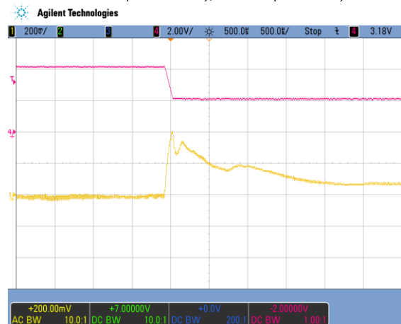
Figure 18: Load transient V1, 244 to 122 A (500 \mu s/div) CH1: V1 (200 mV/div); CH4: I1 (100 A/div)
