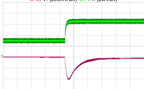
Figure 17 - Load transient V_1 , 30 to 65 A (500 \mu s/div) CH2: V_1 (200mV/div) CH4: I_1 (20A/div)
