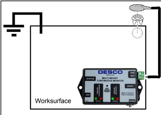
Figure 4. Installation method #1
