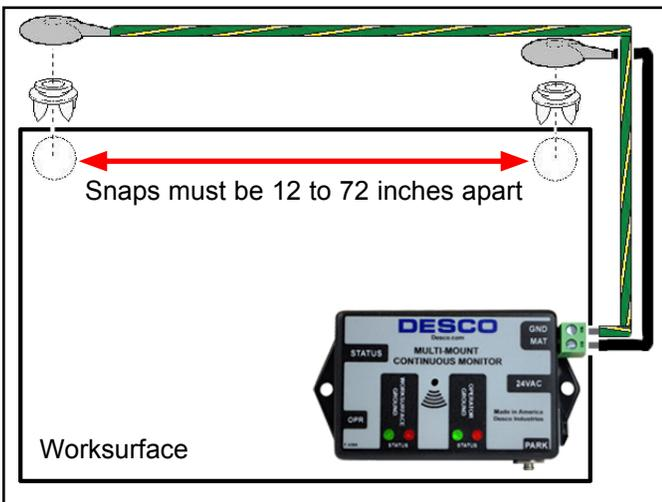
Figure 5. Installation method #2
