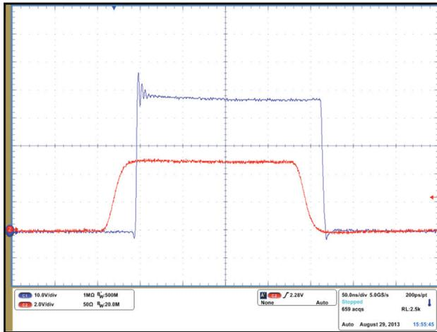
Figure 4: Typical Waveforms for  $V_{IN} = 48\text{ V}$  to  $5\text{ V}/7\text{ A}$  (500kHz) Buck converter
