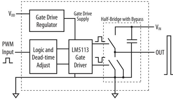
Figure 1: Block Diagram of EPC9002 Development Board
