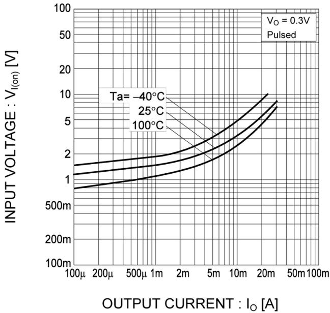
Fig.2 Output Current vs. Input Voltage
