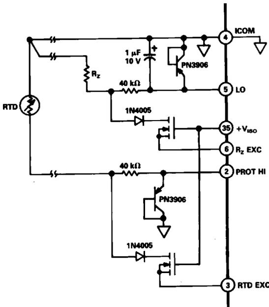
Figure 3. 120 V/240 V AC Normal Mode Input Protection
