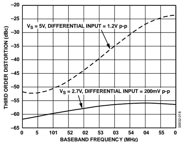
Figure 14. Third Order Distortion vs.  $F_{BB}$
