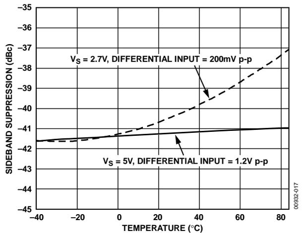
Figure 13. Sideband Suppression vs. Temperature
