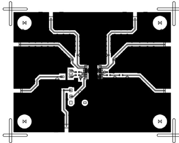
Figure 34. Layout of Evaluation Board, Top Layer
