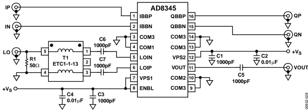
Figure 28. Basic Connections
