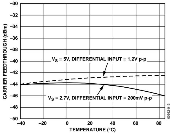
Figure 9. Carrier Feedthrough vs. Temperature
