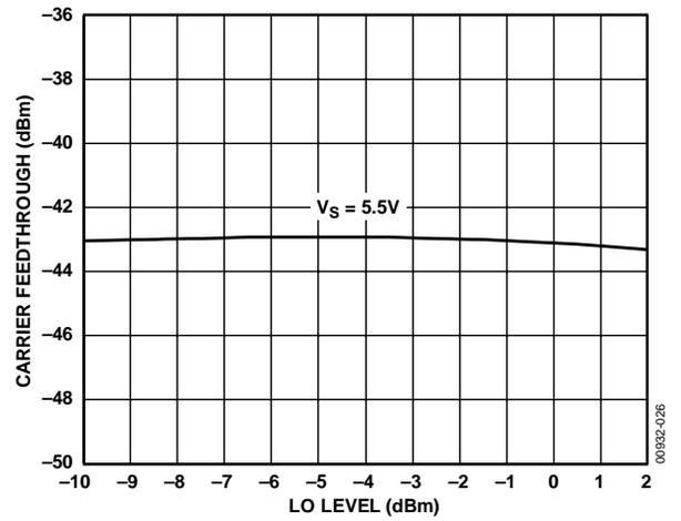
Figure 22. LO Feedthrough vs. LO Input Power
