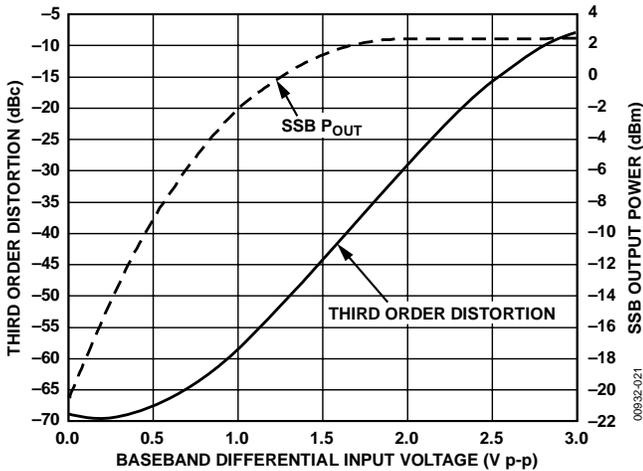
Figure 17. Third Order Distortion and SSB  $P_{OUT}$  vs. Baseband Differential Input Voltage ( $T_A = 25^\circ\text{C}$ ,  $F_{LO} = 800\text{ MHz}$ , LO Level =  $-2\text{ dBm}$ ,  $F_{BB} = 1\text{ MHz}$ ,  $V_S = 5\text{ V}$ )
