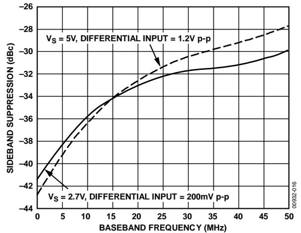
Figure 12. Sideband Suppression vs.  $F_{BB}$
