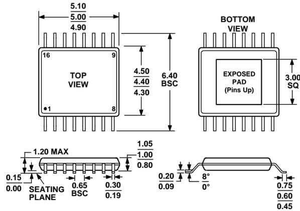
Figure 42. 16-Lead Thin Shrink Small Outline with Exposed Pad (TSSOP\_EP)
