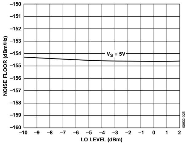
Figure 21. Noise Floor vs. LO Input Power
