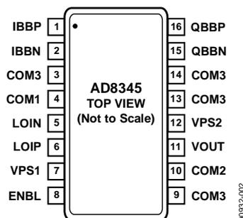
Figure 2. Pin Configuration
