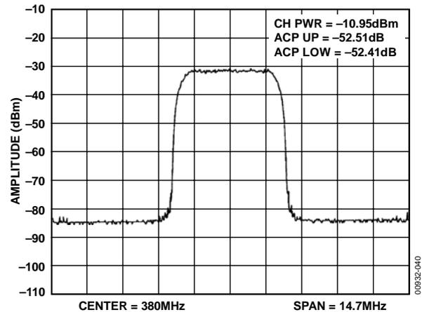
Figure 40. Typical AD8345 WCDMA 3GPP Output Spectrum
