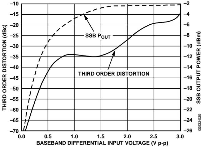
Figure 16. Third Order Distortion and SSB  $P_{OUT}$  vs. Baseband Differential Input Voltage ( $T_A = 25^\circ\text{C}$ ,  $F_{LO} = 800\text{ MHz}$ , LO Level =  $-2\text{ dBm}$ ,  $F_{BB} = 1\text{ MHz}$ ,  $V_S = 2.7\text{ V}$ )
