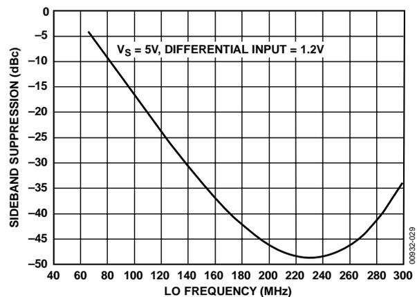
Figure 29. Typical Lower Frequency Sideband Suppression Performance
