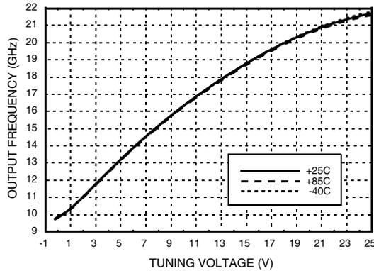
**Frequency vs. Tuning Voltage, T = +25 °C**
