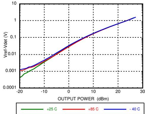
**Detector Voltage vs. Temperature @ 18 GHz**
