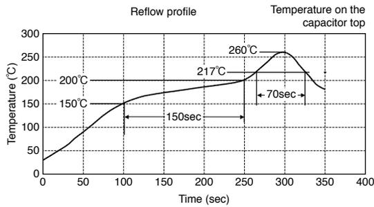
• Above "Reflow Profile" graph indicates temperature at the terminals and capacitor top.
