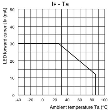
Continuous load current vs. Ambient temperature
