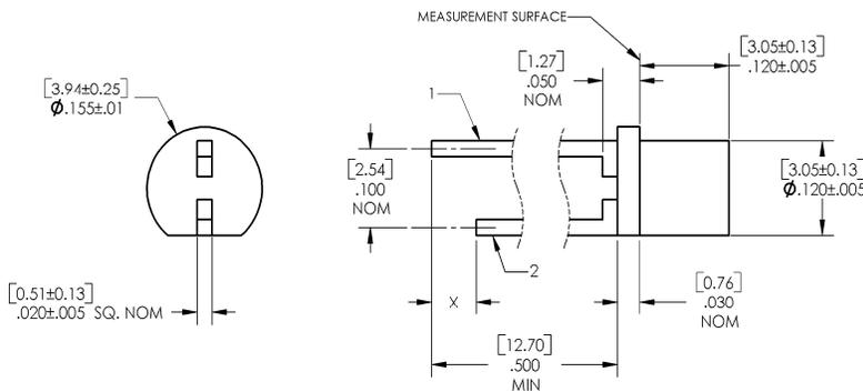
DIMENSIONS ARE IN: [MILLIMETERS]
