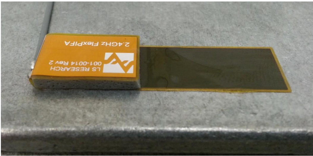
Figure 23 FlexPIFA Mounted on Metal
