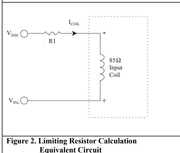
**Figure 2. Limiting Resistor Calculation Equivalent Circuit**
