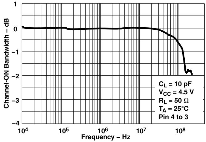
Figure 8. Switch Frequency Response,  $V_{CC} = 4.5 \text{ V}$
