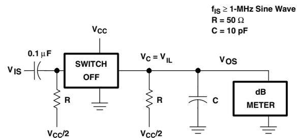
**Figure 5. Switch OFF Signal Feedthrough Test Circuit**
