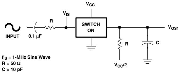
**Figure 1. Crosstalk Between Two Switches Test Circuit**
