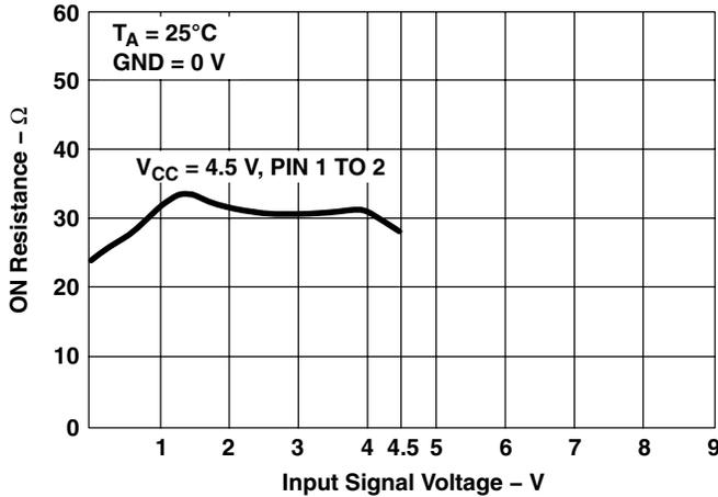
Figure 7. Typical ON Resistance vs Input Signal Voltage
