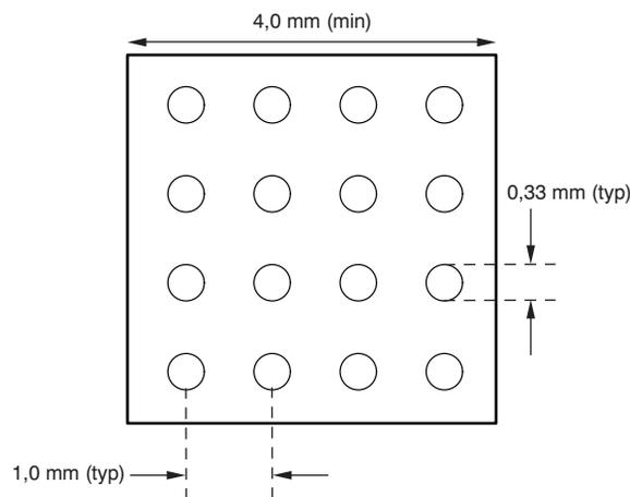
**Figure 20. Recommended PCB Layout**
