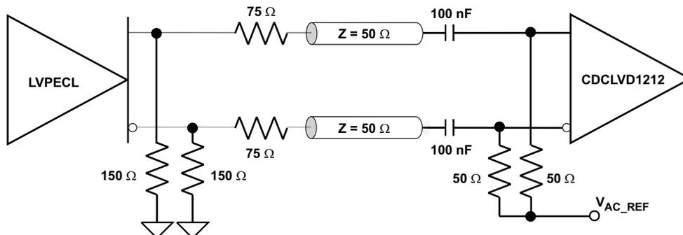
**Figure 14. LVPECL Clock Driver Connected to CDCLVD1212 Input**
