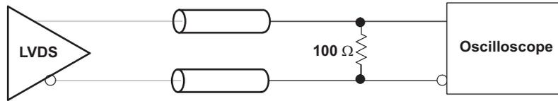
Figure 3. LVDS Output DC Configuration During Device Test
