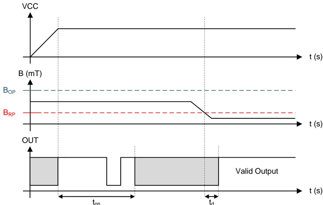
Figure 16. Case 4: Power On When B<sub>RP</sub> < B < B<sub>OP</sub>, Followed by B < B<sub>RP</sub>
