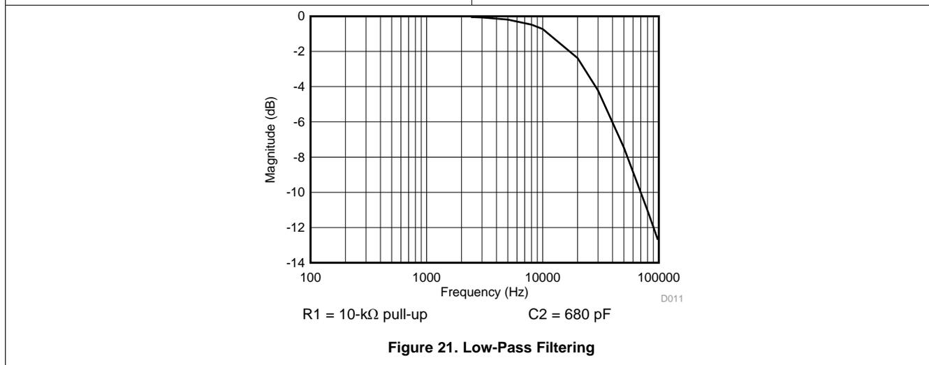
Figure 21. Low-Pass Filtering
