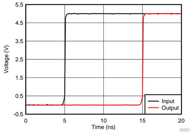
**Figure 1. Simulated Propagation Delay From Input to Output**
