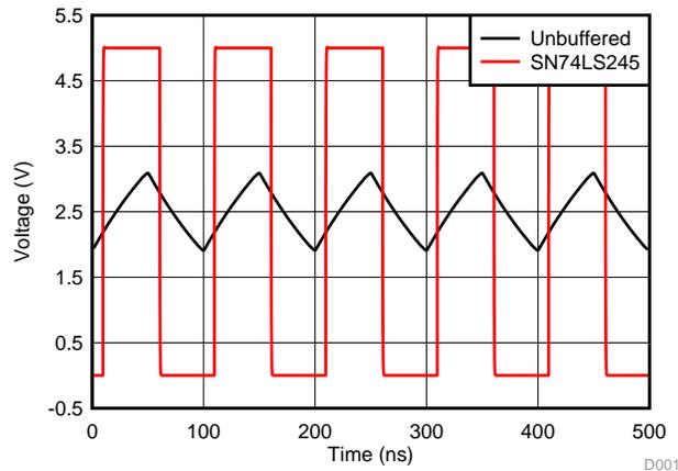
Unbuffered line is directly connected to low current source, SN74LS245 line is buffered through the transceiver. Both signals are measured at the distant end of the ribbon cable. **Input signal is not shown.**
