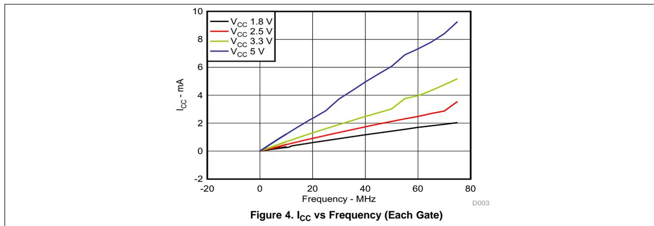
Figure 4. I<sub>CC</sub> vs Frequency (Each Gate)
