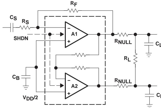
NOTE:  $R_{NULL}$  will reduce the output drive capability of the TLV4120.
