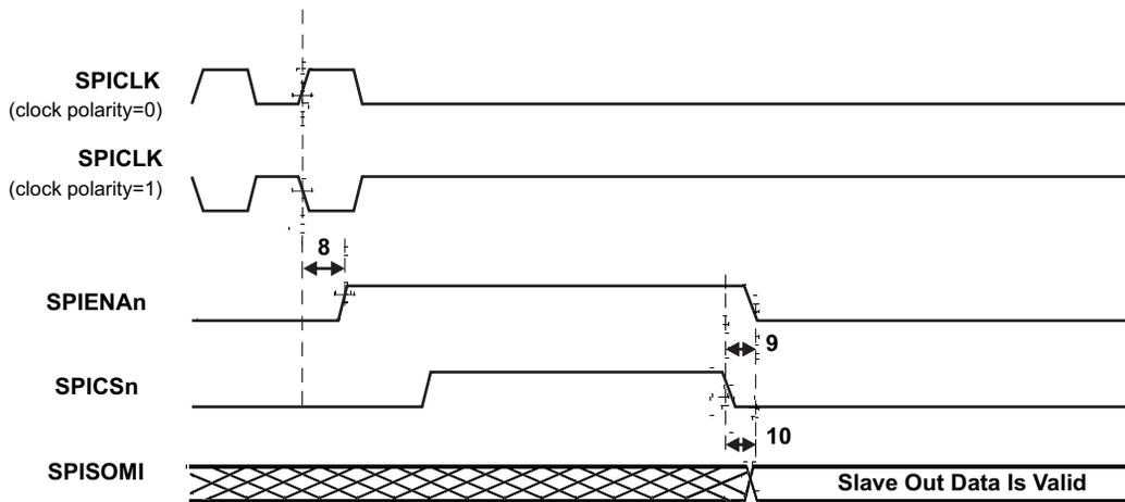
Figure 7-17. SPI Slave Mode Enable Timing (CLOCK PHASE = 1)
