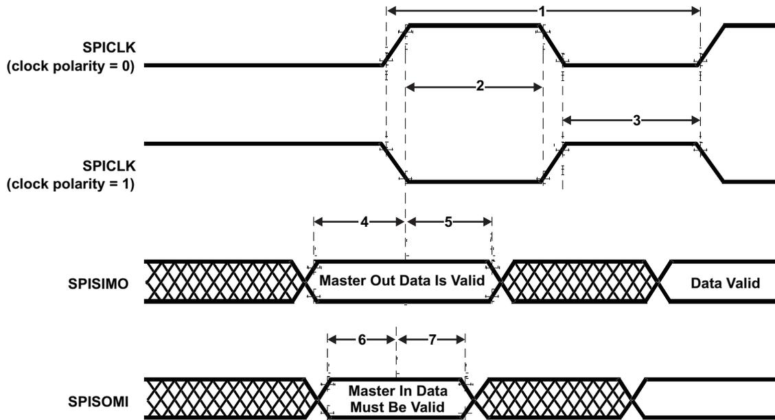
Figure 7-12. SPI Master Mode External Timing (CLOCK PHASE = 1)
