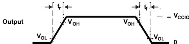
Figure 5-3. CMOS-Level Outputs
