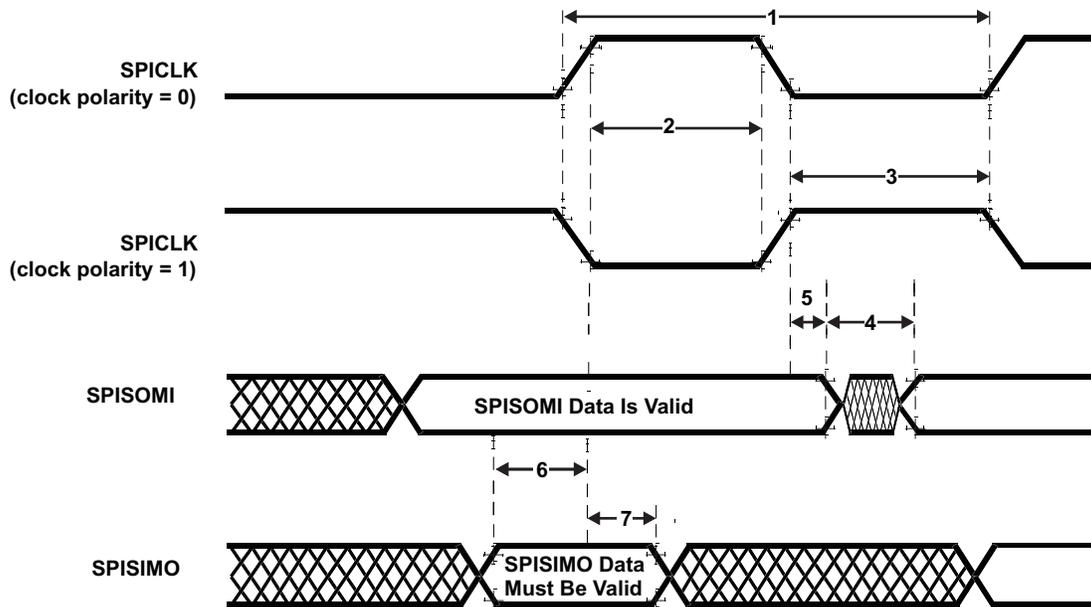
Figure 7-16. SPI Slave Mode External Timing (CLOCK PHASE = 1)
