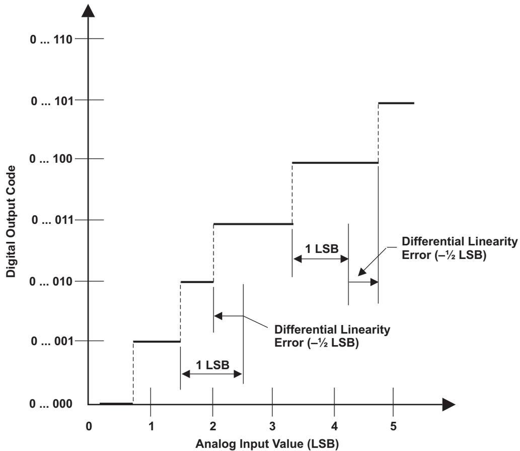
NOTE A:  $1 \text{ LSB} = (\text{AD}_{\text{REFHI}} - \text{AD}_{\text{REFLO}}) / 2^{12}$
