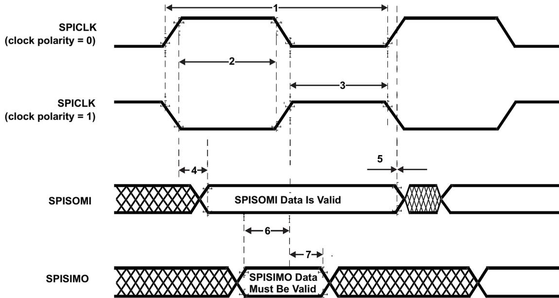
Figure 7-14. SPI Slave Mode External Timing (CLOCK PHASE = 0)
