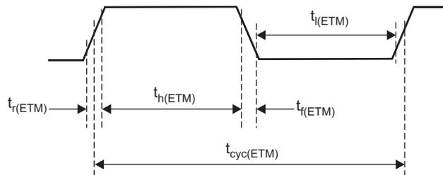
**Figure 6-24. ETMTRACECLKOUT Timing**
