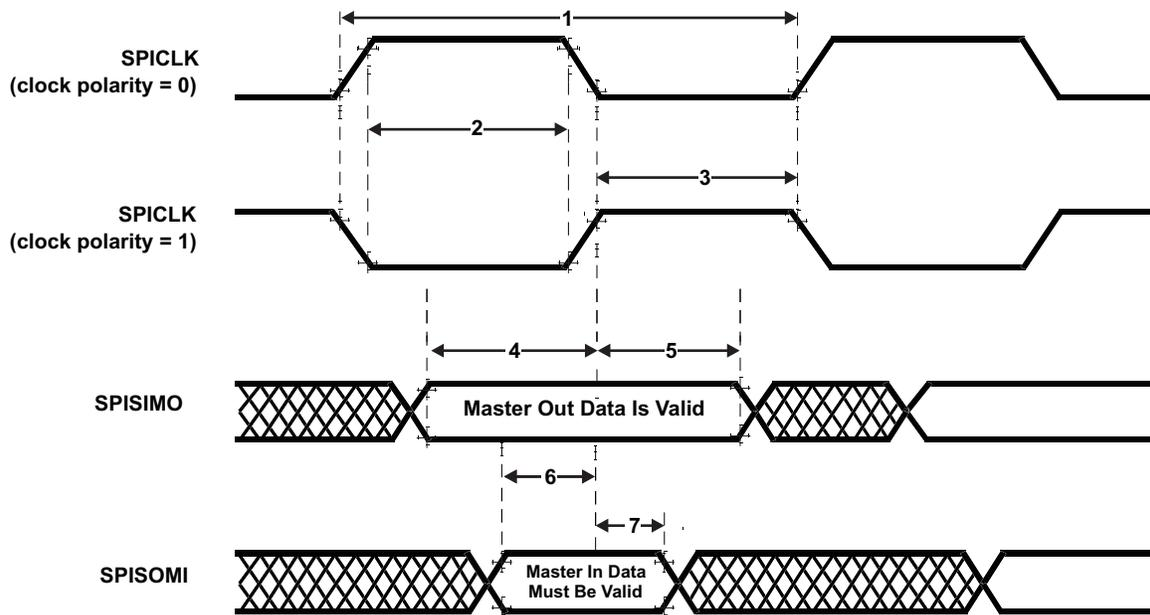
Figure 7-10. SPI Master Mode External Timing (CLOCK PHASE = 0)
