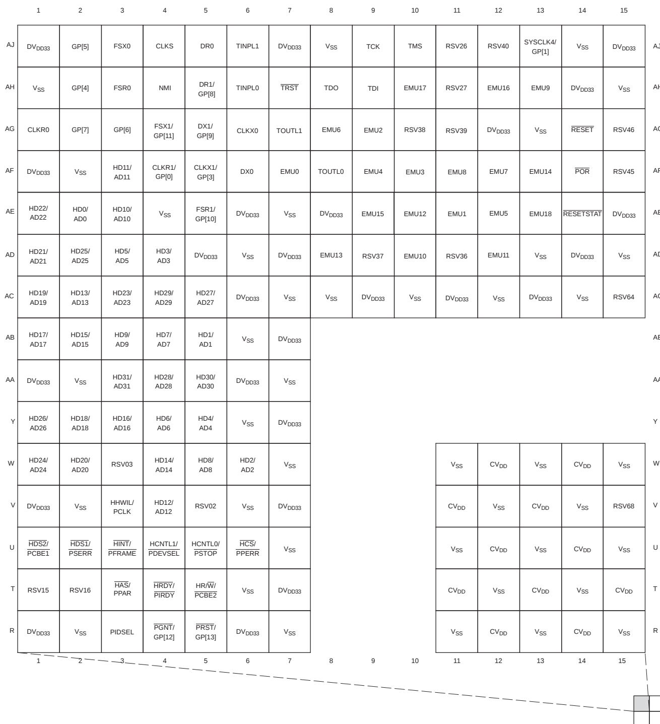
Figure 2-2. C6454 Pin Map (Bottom View) [Quadrant A]
